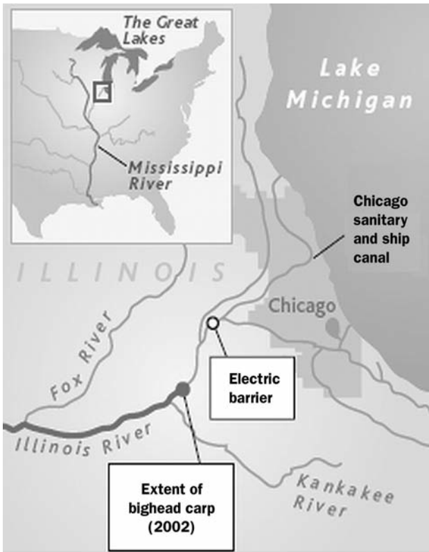
Figure 2. Location of aquatic nuisance dispersal barriers with respect to Asian bighead carp ( Aristichthys nobilis ) distributions in the vicinity of the Chicago Sanitary and Ship Canal. Source: Figure modified from Stokstad (2003).
